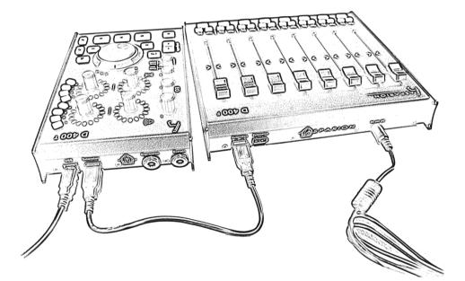
Attention! The connectors for the extensions are no USB connectors. You must never plug in another device there or connect the extension link cable to your computer.
